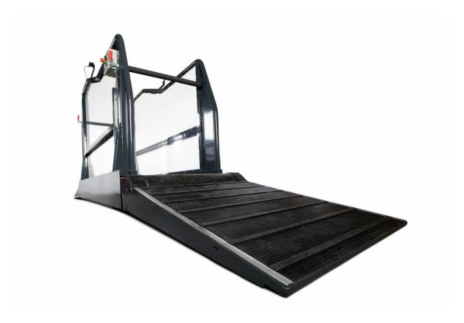
The height adjustment can optionally be built on the treadmill. The hydraulic cylinders are concealed under the side covers and ensure that the treadmill can rise about 6%. By means of 2 push buttons the belt can be angled while the horse is walking on the belt.
