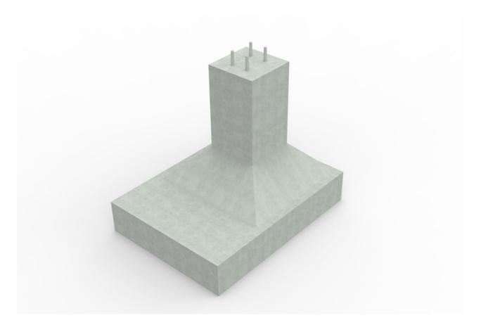
Concretefoot to mount the steel construction of the roof, because of the asymmetrical shape the base provides stability in the construction.
